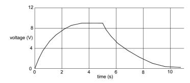
(ii) Delay can be increased by: Increasing the value of C1, 1 mark Increasing the value of R1, 1 mark
