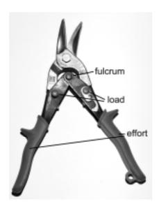
(b) Lever **B** is a pair of **first class** levers, allow '**first order**' levers, 1 mark.
